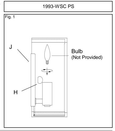
1. Install the light bulbs in accordance with the fixture's specifications.
